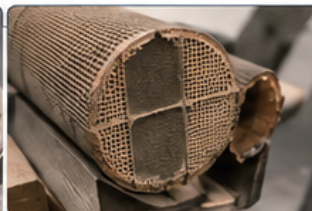
SCR触媒の劣化・閉塞
